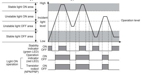
\*\*The waveforms of "Operation indicator" and "Transistor output" are for Light ON, The waveforms are reversed for Dark ON.
